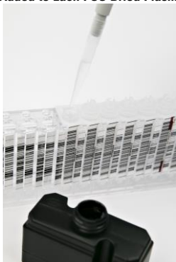
Figure 16 1100 \mu l SPEX Added to Each PSC Dried Plasma Spot Sample
