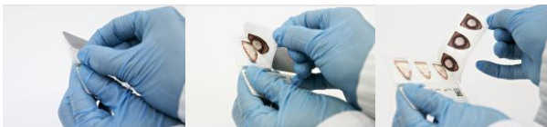
Figure 12 Removal of the PSC Dried Plasma Spot and Bending
