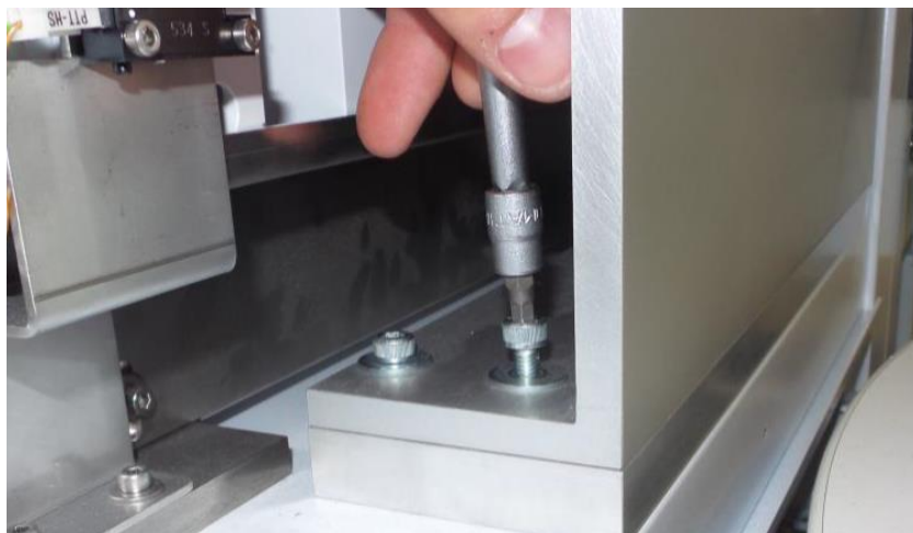
Figure 7: Installing recapper (2 of 2)
