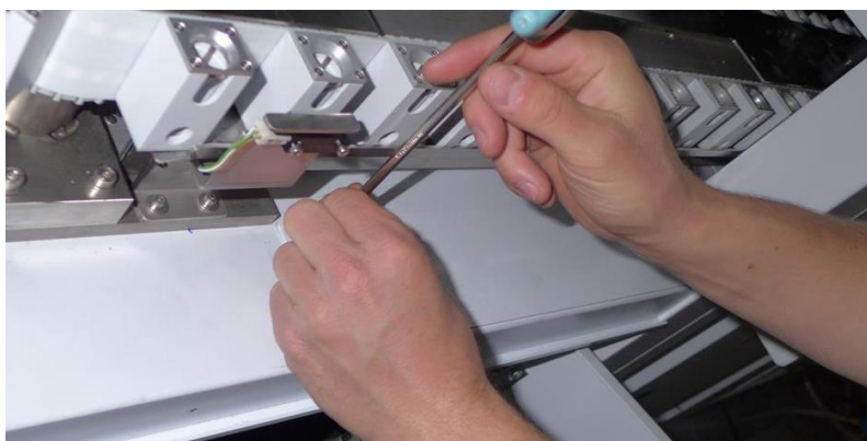
Figure 2: Removing cover panel behind RTT
