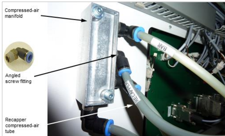
Figure 18: Connecting compressed-air tube
