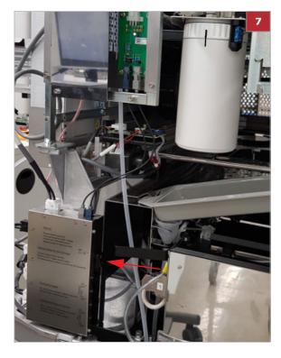
**7** On the PCB voltage selector, switch off the power of the ISE power supply.
