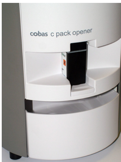
Figure 9 A cobas c pack large jammed in a cobas c pack opener
