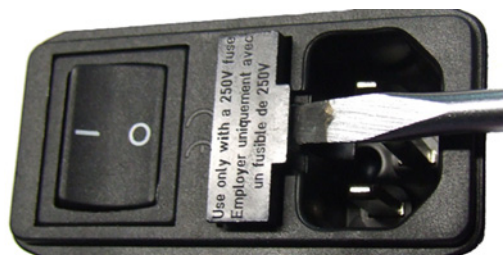
Figure 8 Lifting the fuse holder
