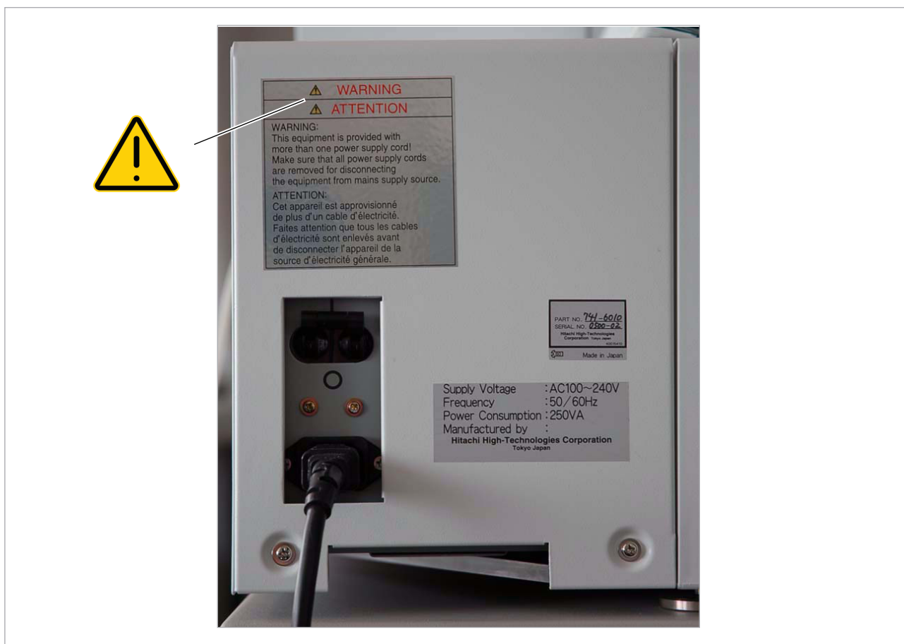
📷 Safety labels on the rack sampler circuit breaker
