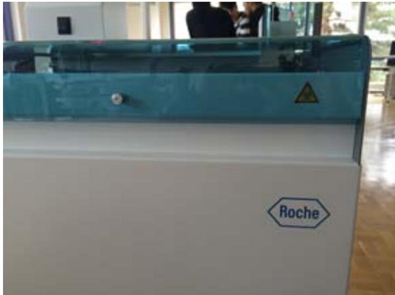
**Figure A-1** Contamination label on front panel of the Liaison® XL Connection Module
