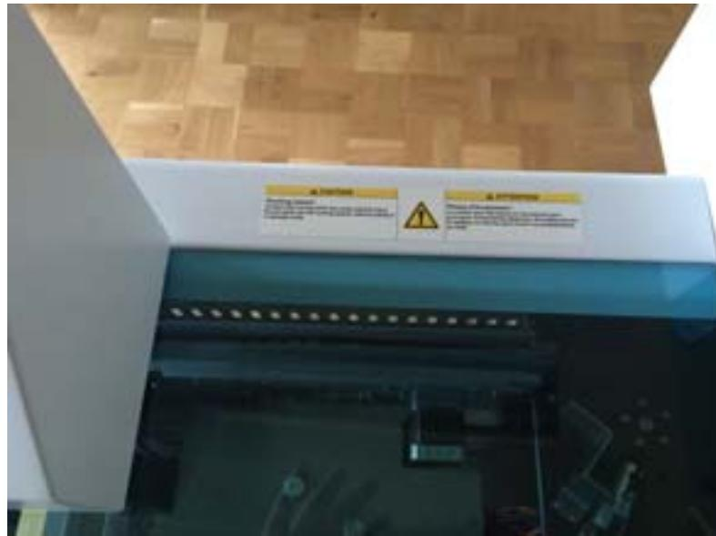
**Figure A-3** Pinching hazard warning label at top of the Liaison® XL Connection Module
