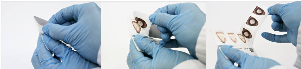
Figure 6 Removal of spotting layer
