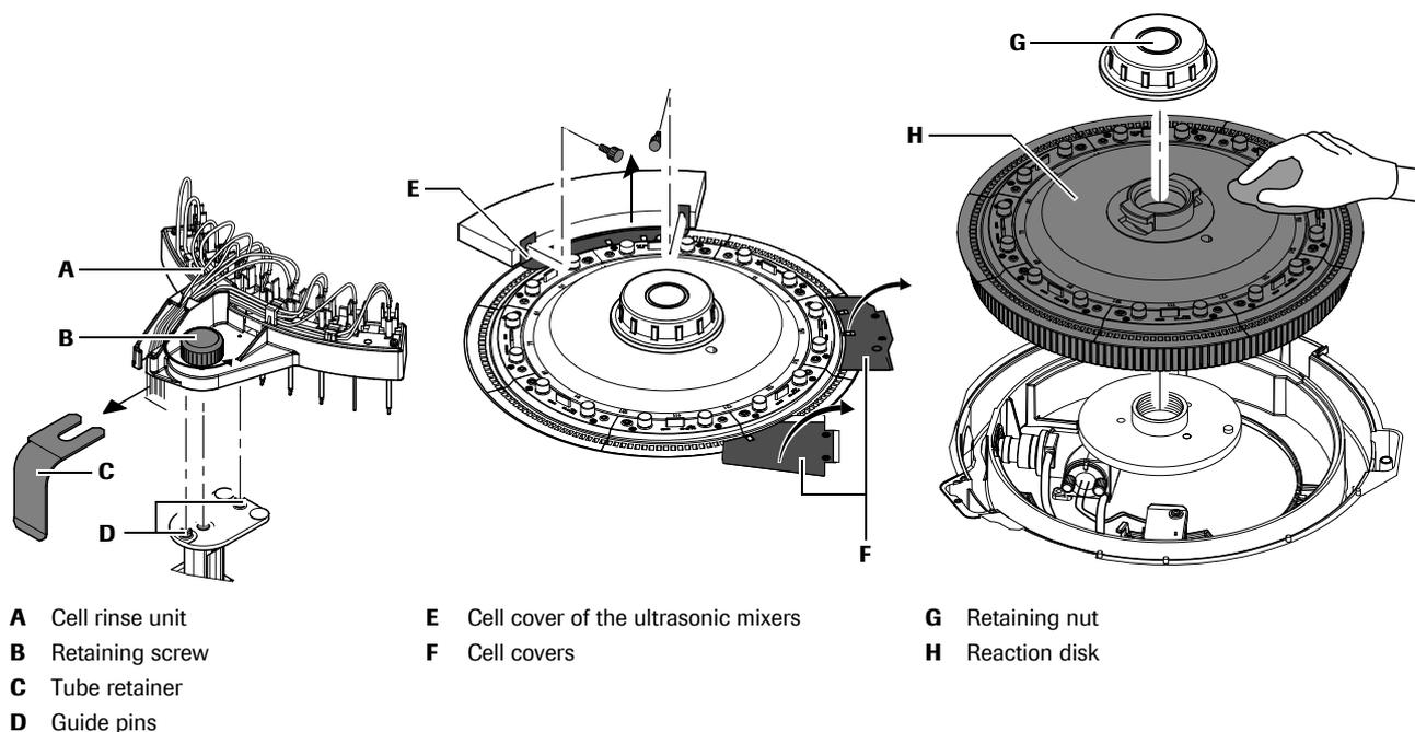
**Figure -2** Dismount the cell rinse unit and the reaction cells
