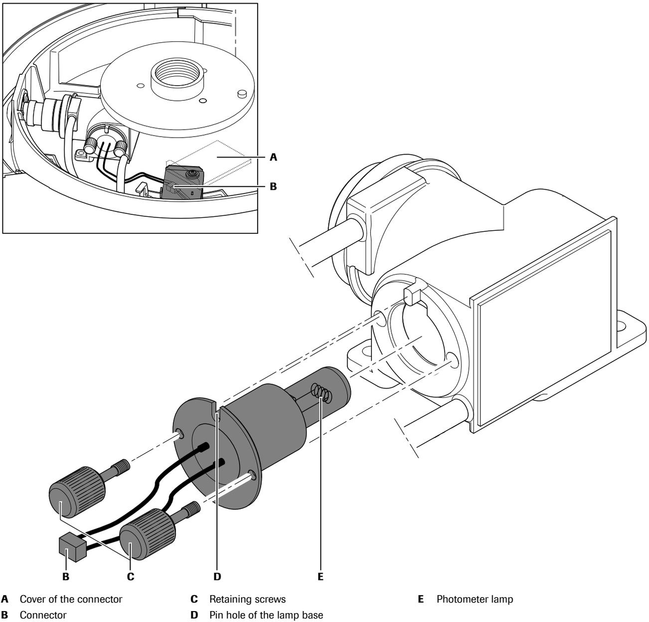
**A** Cover of the connector      **C** Retaining screws      **E** Photometer lamp
