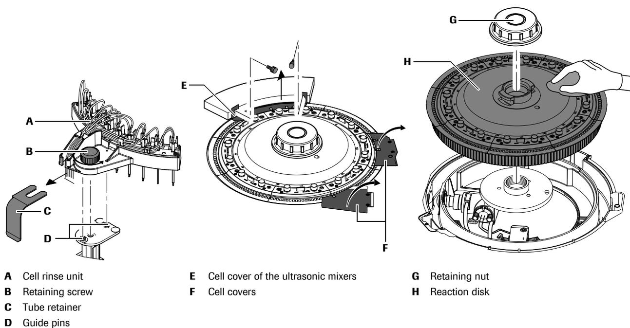
**Figure -8** Dismount the cell rinse unit and the reaction cells
