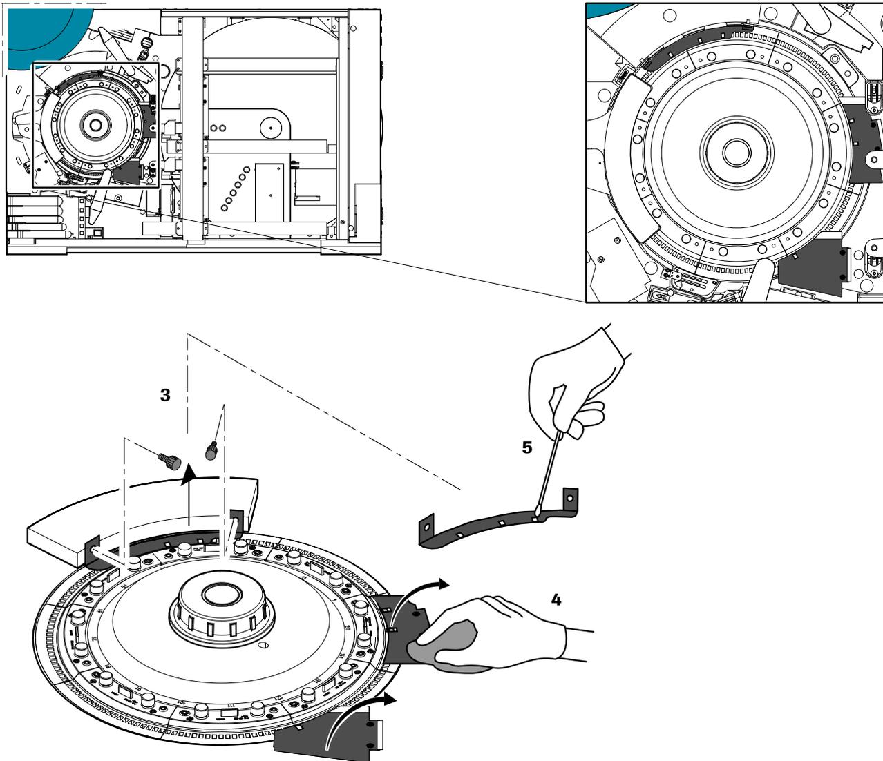
**Figure -1** Cleaning the cell covers
