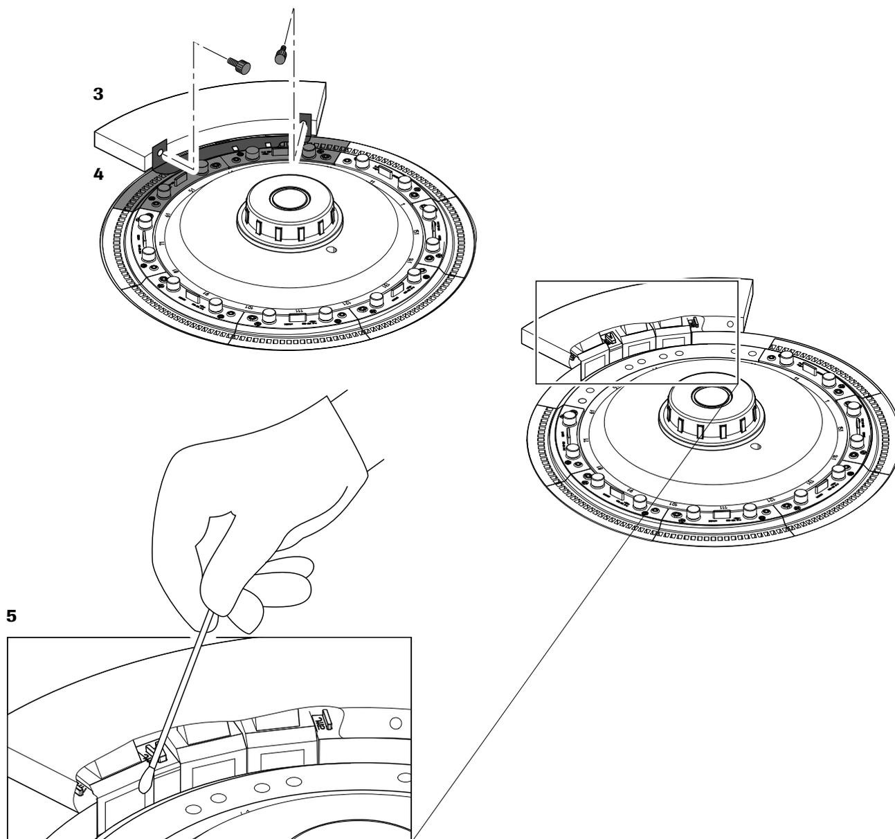
**Figure -6** Cleaning surface of ultrasonic mixer with cotton swabs
