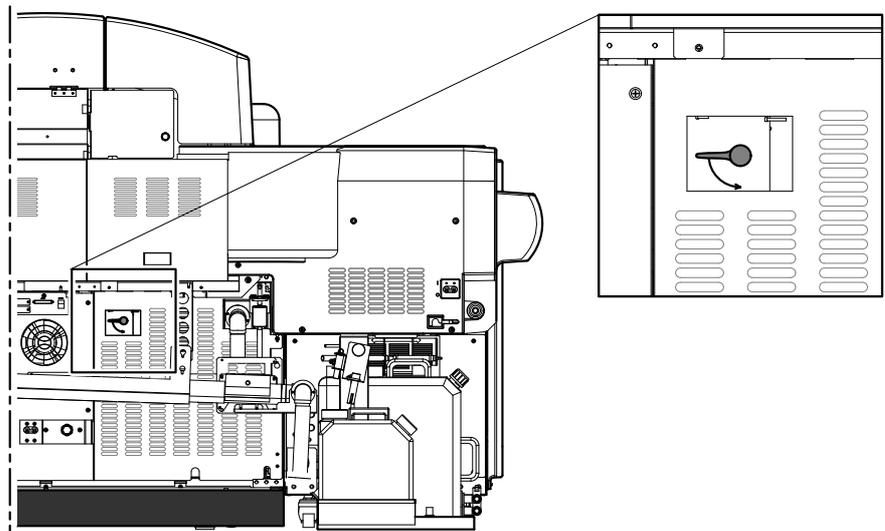
**Figure -4** Tap for manually draining the incubator bath
