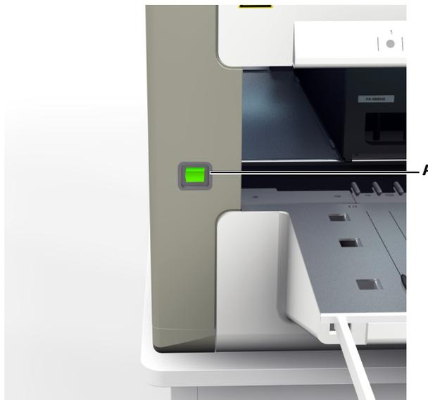
A Power switch of the instrument
