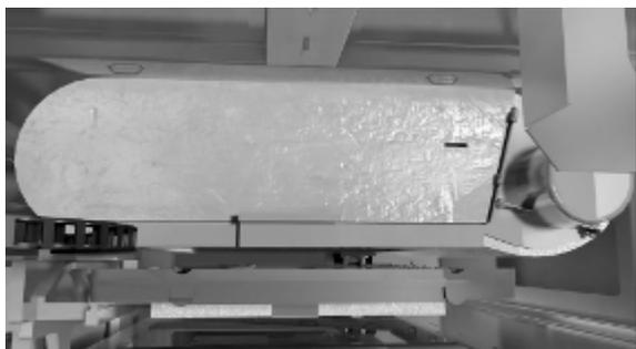
The curing oven cures coverslip glue and helps remove residual fluid from the slide tray.
