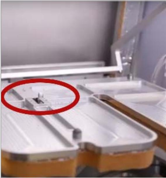
These photos show the switch sensor on the slide dryer door.
