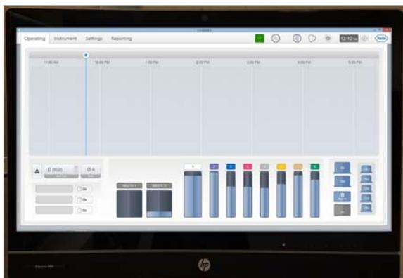
The touch screen monitor is integrated with the computer. The monitor is mounted on the right side of the system and can swing left and right or tilt back and forth for easy access. Use your finger to navigate and select information or use the available keyboard to interact with the user interface.
