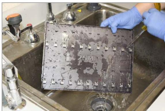
**1** Clean the tray using deionized water only. Do not use a dishwasher to clean trays.
