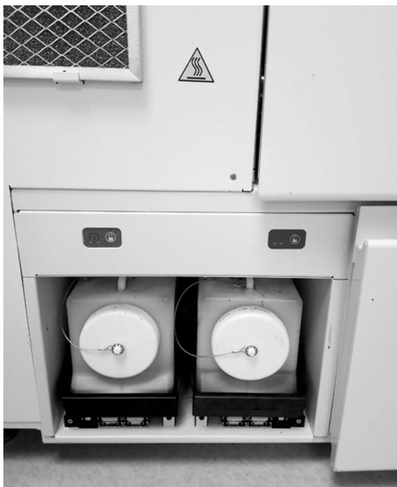
The VENTANA HE 600 system can collect liquid waste in waste containers or direct the waste to the drain.
