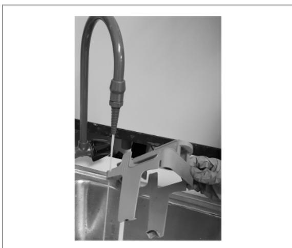
2 Wash the reagent hat and tubing with deionized water. Allow to dry.
