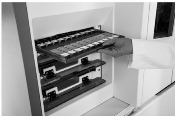
Trays are loaded into tray portals to begin slide processing and unloaded from portals when processing is complete.
