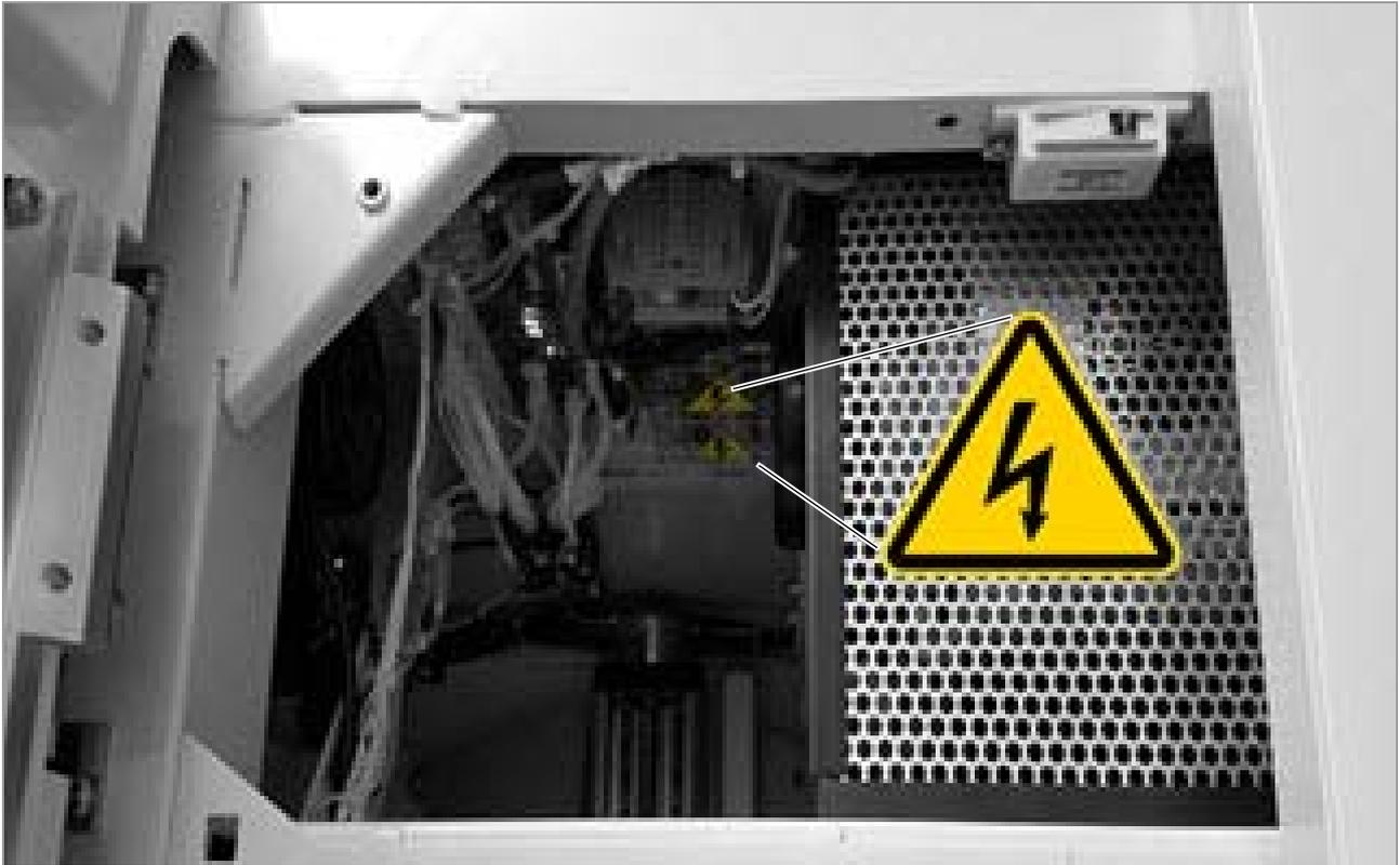
☒ Safety labels on the top of the transportation system module (bottom view)
