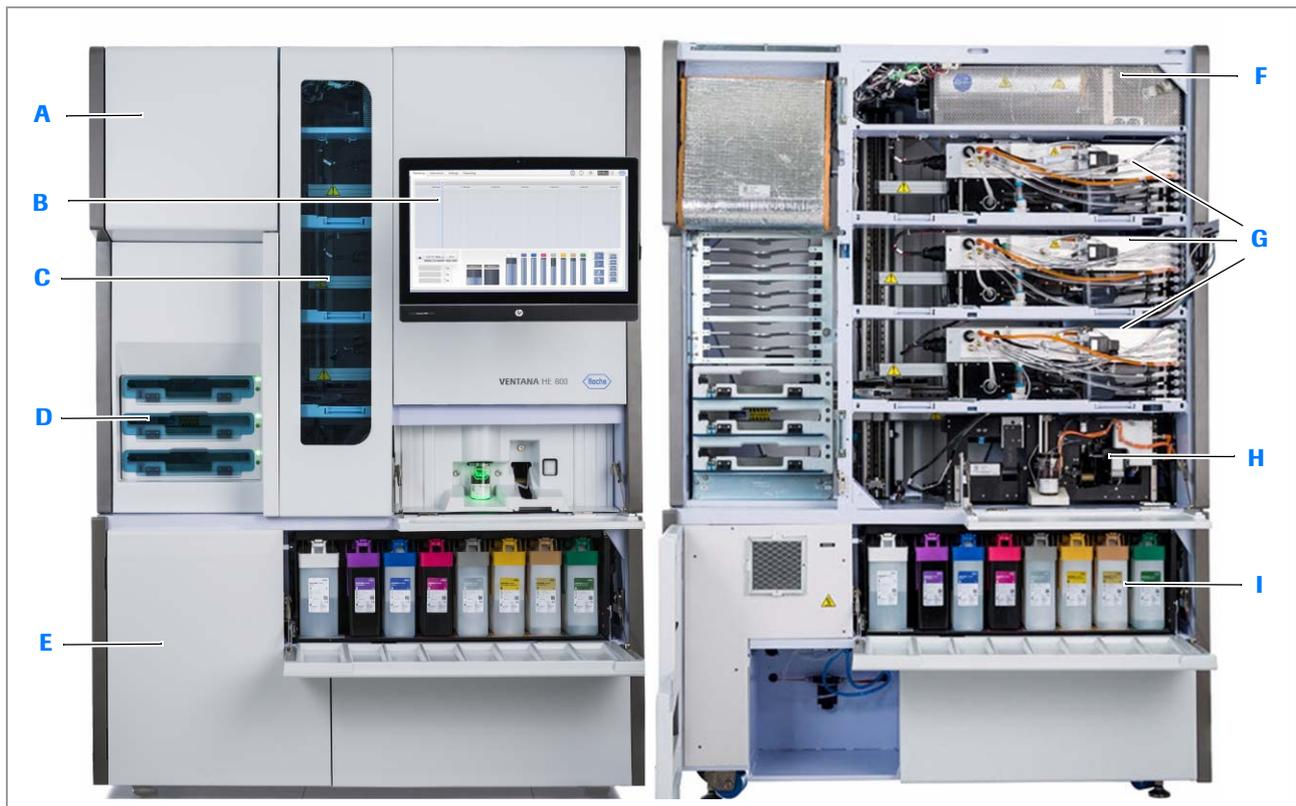
**A** Slide dryer (drying oven)
