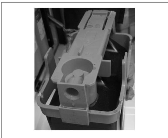
**3** Check to see if fluid is present in the reagent drip trap on the back of the hat.
