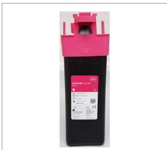
Reagents are shipped and stored in disposable bottles with colored and numbered labels. Those labels match the color and number on the reagent hat assembly and on the **Operating** tab status indicator.
