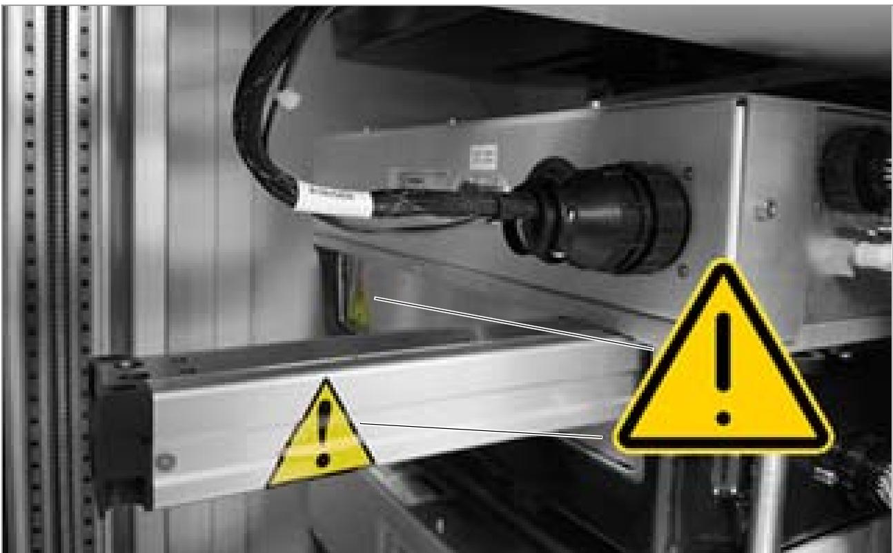
☒ Safety labels on each arm of the stainer crank and door in the transportation system module
