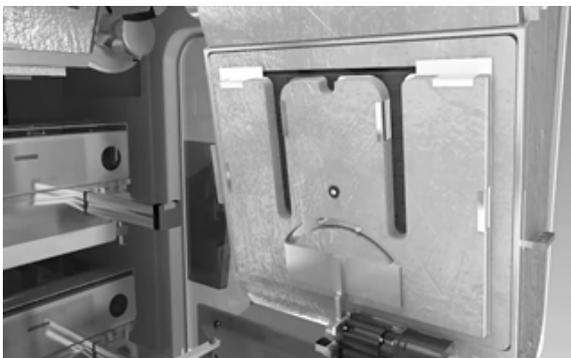
The slide dryer tilts the slide tray at an 80° angle to drain moisture from the slides. The tray is then heated in the oven at a temperature range of 72 °C +/- 3 °C.
