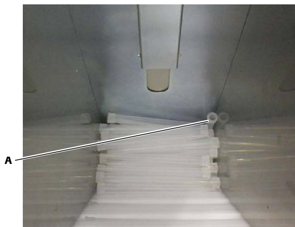
Figure 20 A tip causing a blockage in the tip container
