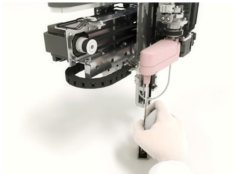
**Figure 23-3** Cleaning the outside of the c 701 / c 702 sample probes
