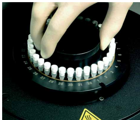
G) Transferring the LightCycler® 2.0 Sample Carousel into the LightCycler® 2.0 Instrument.
