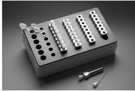
C) The LightCycler® Centrifuge Adapters within cooling block.
