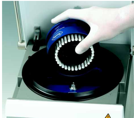
E) Inserting the LightCycler® 2.0 Sample Carousel within the centrifuge bucket into the LC Carousel Centrifuge 2.0.
