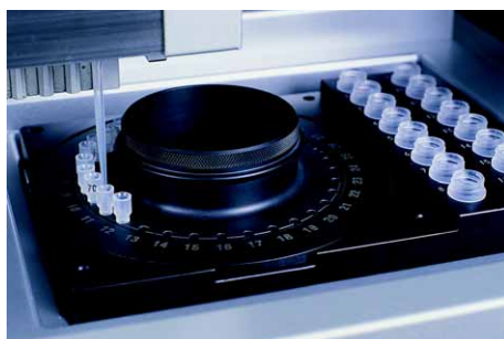
B) The MagNA Pure LC Cooling Block, LC Sample Carousel with the LightCycler® Sample Carousel assembled.
