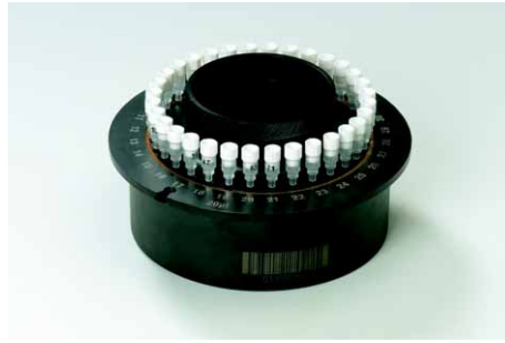
D) The LightCycler® 2.0 Sample Carousel with filled and sealed capillaries inserted.
