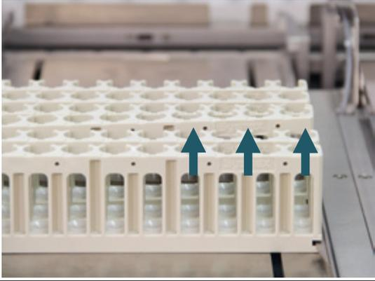
A close-up photograph showing a white plastic rack being inserted into a metal guide rail. Three blue arrows point upwards from the top surface of the rack, indicating it is being pushed onto the rail instead of being inserted from the side. | <b>X</b>  |
