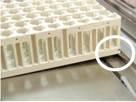
A close-up photograph showing a white plastic rack being inserted into a metal guide rail. The rack is tilted to the right. A white circle highlights the bottom notch, which is not properly seated in the rail's groove.                         | <b>X</b>  |
