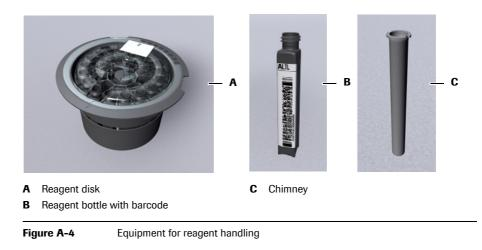
*Reagent disk* On the instrument, the reagents are stored on a reagent disk. It provides space for 27 bottles, allowing up to 14 reagent sets to be installed on the disk, assuming that most tests need two reagents. Extra diluents and cleaners are also loaded on the reagent disk.
