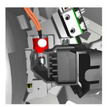
Hold the assembly by the screw and fit the lamp socket in the guides.
