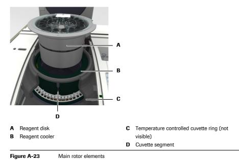
Rotational movement The bottles and cuvettes are positioned in a manner that they can be moved to the various positions by a rotational movement. There are positions for loading and removal (reagent and cuvette ports), pipetting, and measuring.
