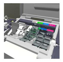
**9** On the screen, press the electrode button to confirm that you have removed the electrode.
