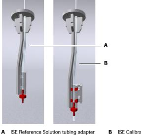
**B** ISE Calibrator indirect/urine tubing adapter
