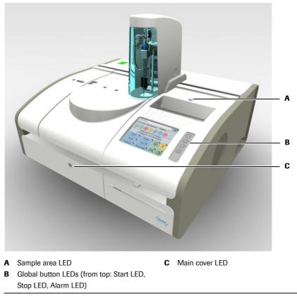
Figure A-86The Cedex Bio instrument
