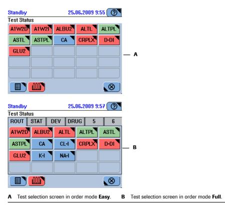
Figure A-53 Test selection screen
