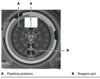
Figure A-24 Reagent port on the reagent disk
