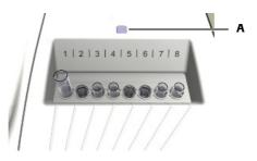
**A** The LED indicates that the transfer tower is approaching or that you should place a sample tube.
