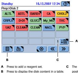
The number indicates the number of free Press to display the disk content in a table. positions on the disk.
