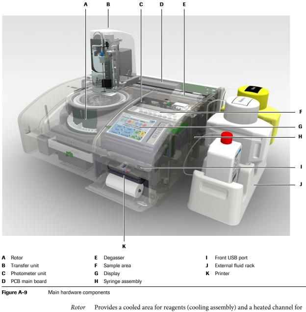
The following figure illustrates the main components of the Cedex Bio instrument.
