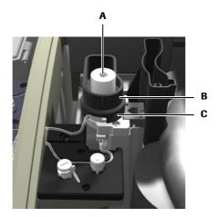
• Remove the ISE overflow collector (B) by pulling it upwards and turning it from side to side as you do so.
