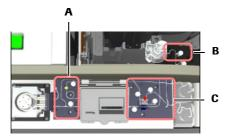
Removing the pinch valve caps and clamps
