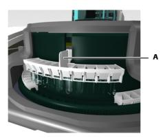
**A** Hold the segment by its handle. Make sure not to touch the cuvettes.
