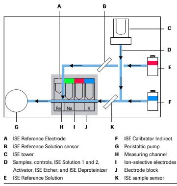
Figure E-1 Main parts of the ISE measuring system
