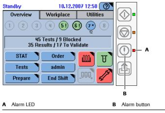
Figure D-2 Alarm LED
