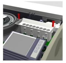
Removing the rotor
