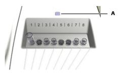
A Sample area LED. A green LED indicates that you should place a tube, a blinking yellow LED that you should keep clear of the sample area.
