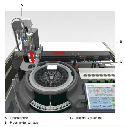
Figure A-15 Major elements of the robotic transfer unit
