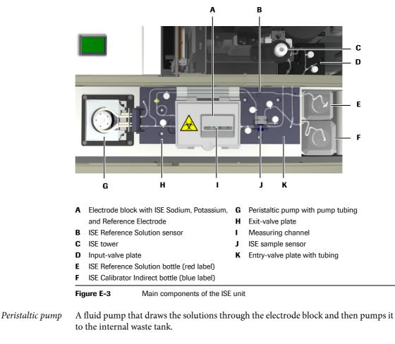
*Input-valve plate* A set of valves to create cleaning segments and to control the flow of waste fluids.
