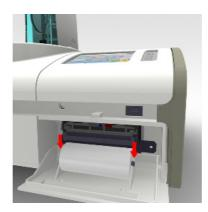
7 Insert the paper in the slot in the printer panel and pull some through.
