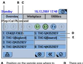
A Position on the sample area where to place the calibrator.
