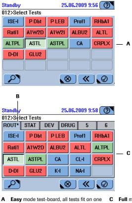
**Full** mode test-board. The tests are distributed across several panels (tabs).
