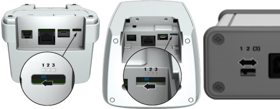
Fig 3-1 USB Configuration Switch positions on HBU (left), BU (middle) and BUH (right)
