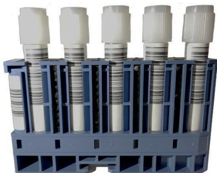
Figure 1 Correct placement of sample tubes in MPA rack prior to sonication
