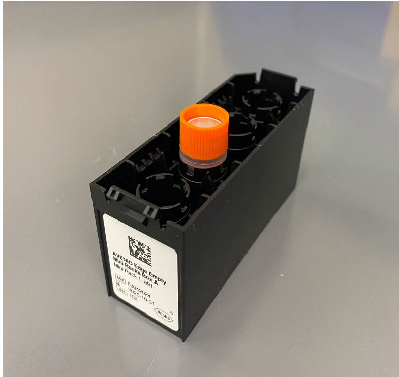
Figure 5: Reagent mini rack preparation. Tube is placed into reagent mini rack position 1. Positions 0, 2, and 3 are empty.
