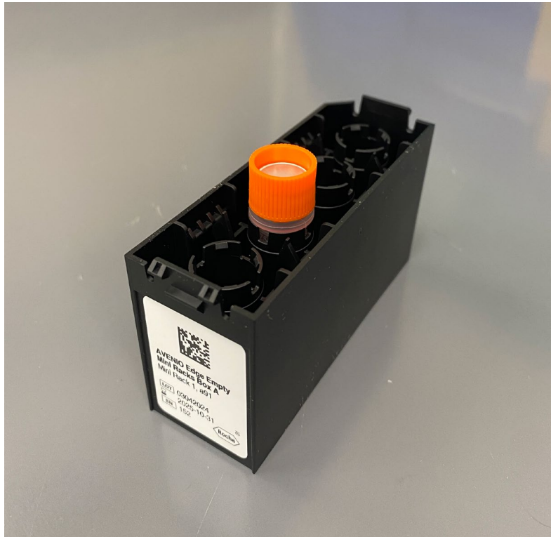
Figure 3: Reagent mini rack preparation. Tube is placed into reagent mini rack position 1. Positions 0, 2, and 3 are empty.
